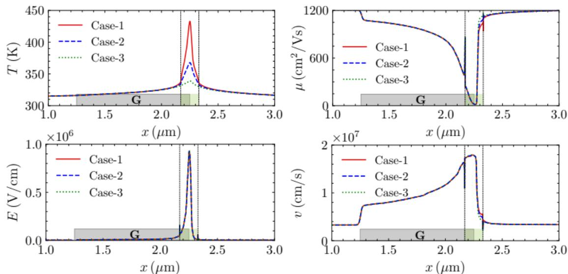
**Figure 13:** Channel temperature, electron velocity, electric field, and electron mobility distributions at  $V_g = -1 \text{ V}$ ,  $V_d = 6.7 \text{ V}$ .
