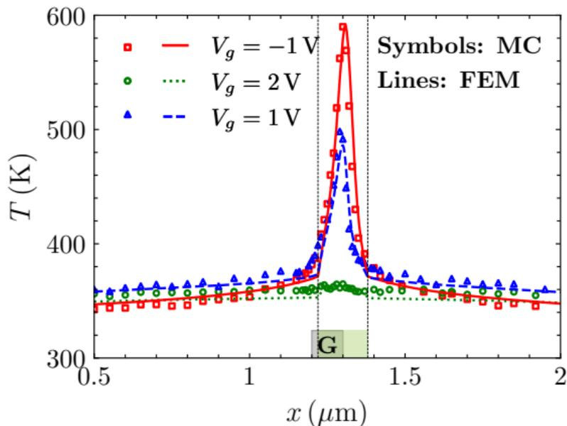
Figure 10: Comparison of channel temperature distributions predicted by MC simulation and FEM with  $k_{\text{eff}}$  at different biases with  $P_{\text{diss}} = 5 \text{ W/mm}$ .
