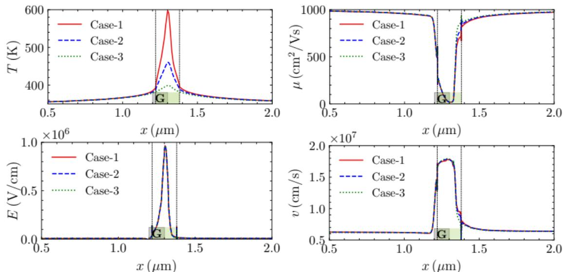
**Figure 11:** Channel temperature, electron velocity, electric field, and electron mobility distributions at  $V_g = -1$  V,  $V_d = 6.7$  V.
