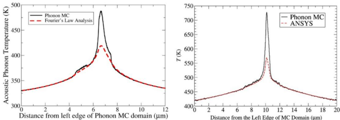
**Figure 1:** Comparison of channel temperature between phonon MC simulation and Fourier's law calculation<sup>12</sup>.
