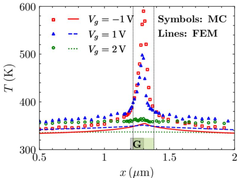
**Figure 8:** Comparison of channel temperature distributions predicted by MC simulation and FEM with  $k_{\text{bulk}}$  at different biases with  $P_{\text{diss}} = 5 \text{ W/mm}$ .
