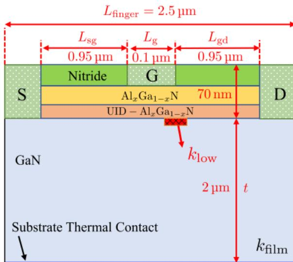
Figure 9: Schematic of channel temperature reconstruction.
