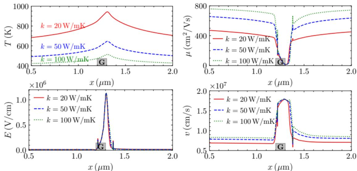
**Figure 15:** Channel temperature, electron velocity, electric field, and electron mobility distributions at  $V_g = 0\text{ V}$ ,  $V_d = 10\text{ V}$ .
