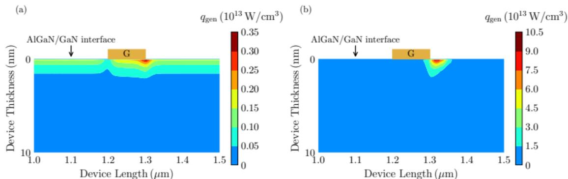
**Figure 3:** Heat source distributions at different biases with  $P_{diss} = 5 \text{ W/mm}$ , (a)  $V_g = 2 \text{ V}$ ,  $V_d = 3.8 \text{ V}$ , (b)  $V_g = -1 \text{ V}$ ,  $V_d = 6.7 \text{ V}$ <sup>4</sup>.
