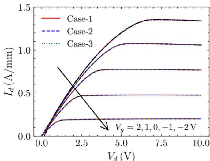
Figure 14: Output characteristics at different biases.
