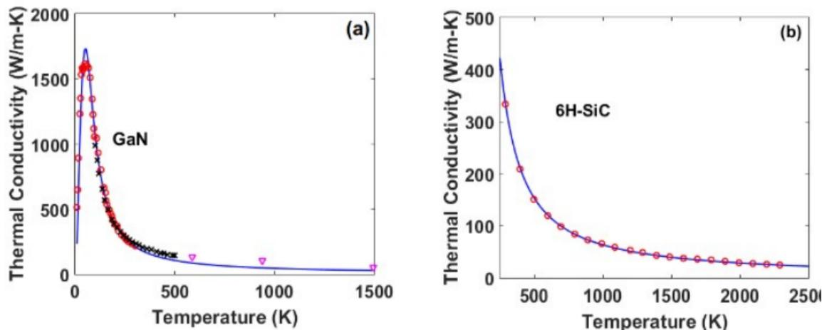
Figure 7: Thermal conductivity from model calculations (line), and from experiments (symbols)<sup>8</sup>.
