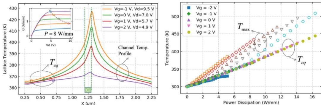
Figure 17: Left: channel temperature profiles at four different biases. Right: Equivalent channel temperature and maximum channel temperature versus the power dissipation.
