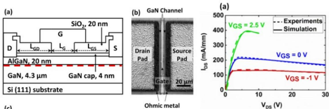
Figure 4: Left: Schematic cross-sectional view of the symmetric AlGaIn/GaN HEMT,  $L_G = 2 \mu\text{m}$ ,  $L_{GS} = L_{GD} = 3 \mu\text{m}$ . Right: Output characteristics of the AlGaIn/GaN HEMT. Test data and simulation show excellent agreement.<sup>5</sup>
