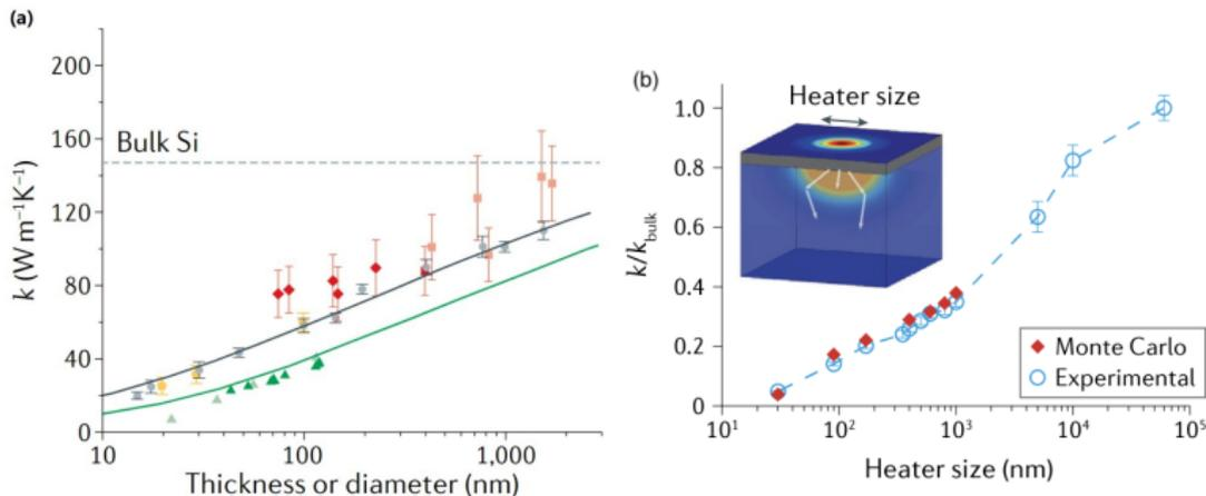
**Figure 2:** (a) Thermal conductivity versus film thickness or nanowire diameter. (b) Effective conductivity versus varying heater sizes<sup>3</sup>.
