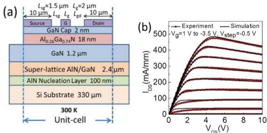
Figure 5: (a) Schematic of lateral AlGaN/GaN HEMT structures on Si substrates. (b) Comparison between simulation and experiment DC output characteristics of a single finger lateral HEMT<sup>6</sup>.
