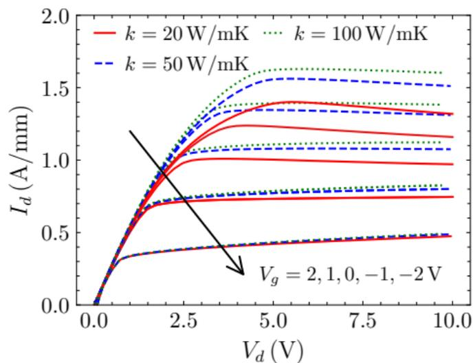
Figure 16: Output characteristics at different biases.
